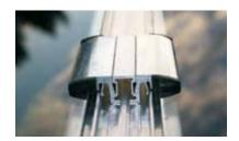
The cross beam always presents a profile geometry that is aligned to the flow of forces (Schletter utility model protection). Thus, the required structural characteristics are achieved with minimum utilization of materials. Mounting grooves are incorporated into all profiles to facilitate assembly. The cross beams are fastened to the supporting units by means of special mounting claws
