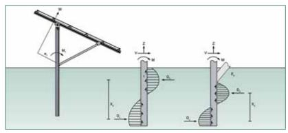
Hot-dip galvanized pile-driven profiles in different size categories are used for the foundation. The custom-developed ram form ensures optimal anchoring in the ground with maximum flexural rigidity. The anchoring forces can also be transmitted as far as the upper connection point, thus ensuring optimal structural safety of the plant and protection against wind and snow loads.
